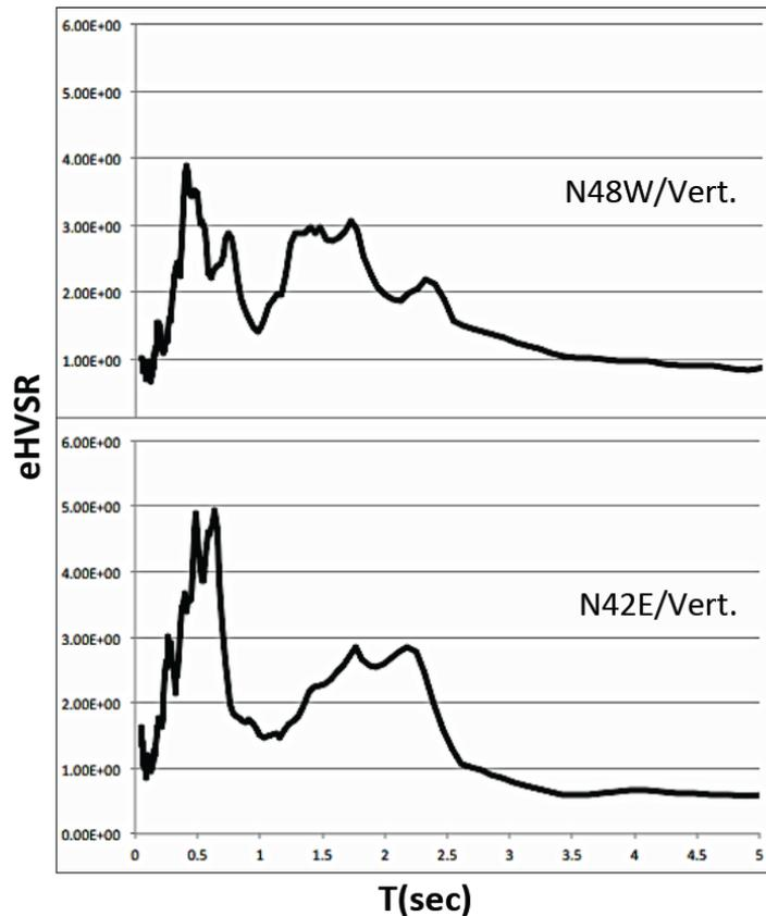
**Fig. 10.** Earthquake Horizontal-to-Vertical spectral ratio for both horizontal components based on the 5% damped response spectra at the SMG1 station.
