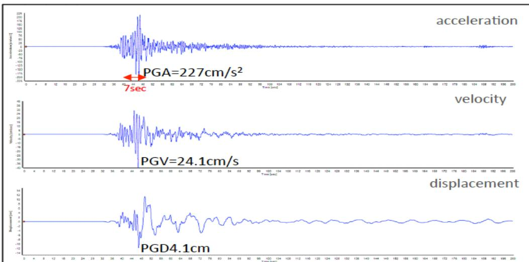
Fig 5. Time histories of the horizontal component (direction N42E).
