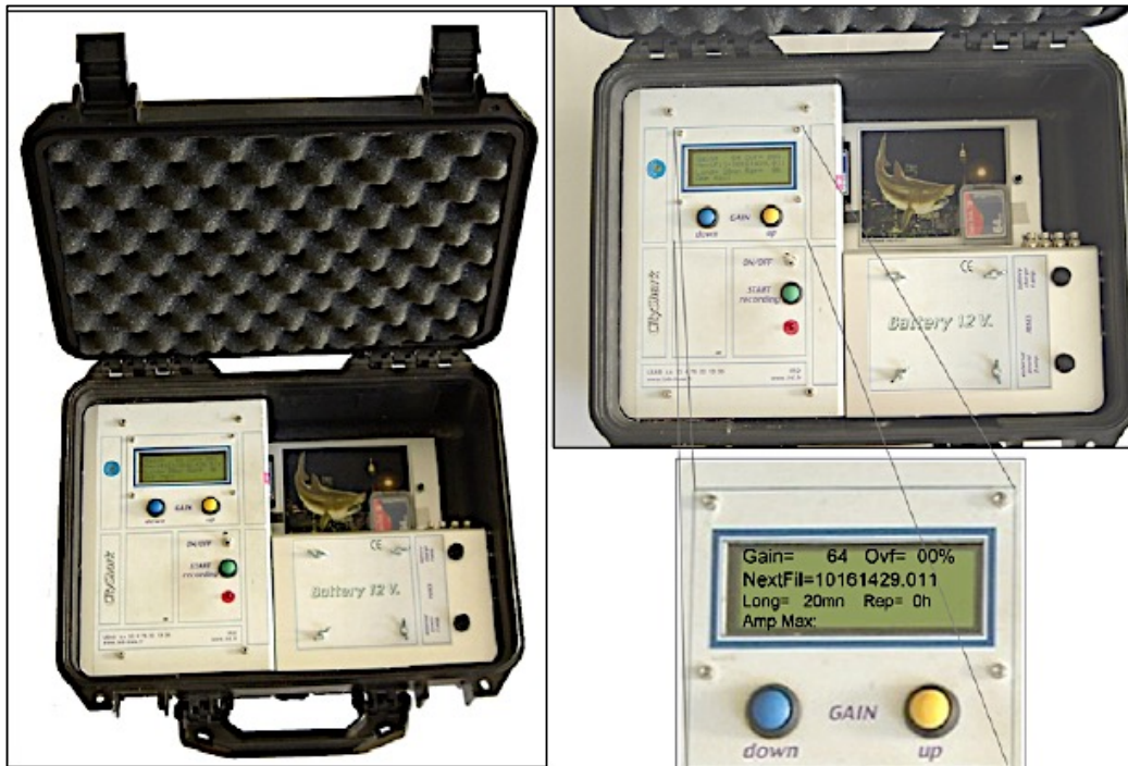
Fig. 1. The CityShark datalogger used for ambient noise measurements in Durres city.
