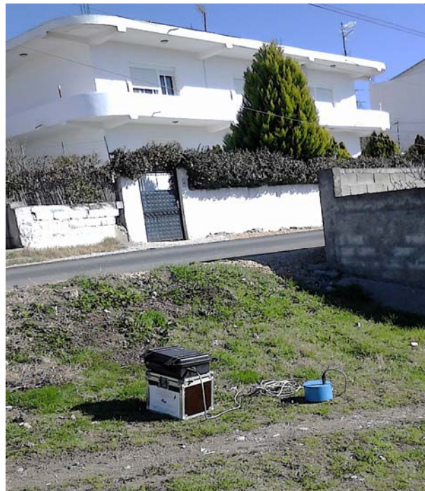
Fig. 4. Typical ambient noise measurement installation (ground coupling) in Durrës city.
