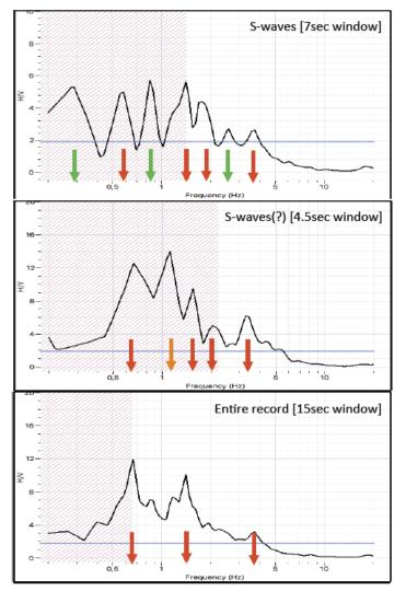
**Figure 13.** Horizontal-to-Vertical Spectral Ratio (HVSR, Receiver Function) at the DURR station estimated for the first S-wave window(upper), the second S-wave(?) window (middle) and the entire record length of the mainshock (down).
