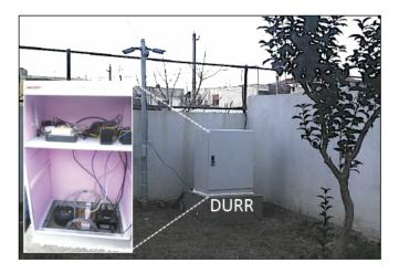
Figure 5. DURR free-field accelerometric station (CMG-DM24).
