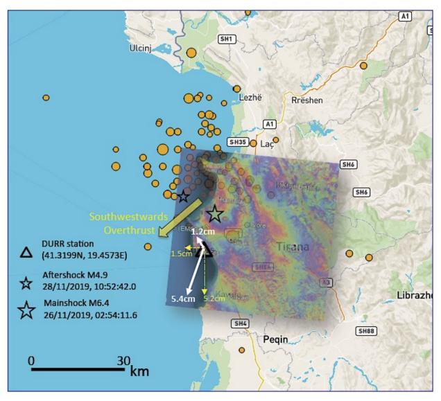
**Figure 10.** Horizontal and vertical permanent displacements (white arrows) estimated from the acceleration time history of Durres (DURR station); two weeks aftershock activity (AUTh Seismological Station & EMSC); interferogram for the mainshock (Tsironi and Ganas 2019).
