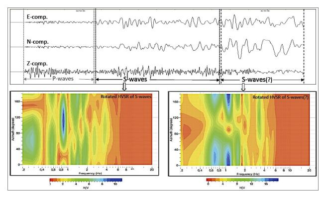
**Figure 12.** Horizontal-to-Vertical Spectral Ratio (HVSR, Receiver Function) at the DURR station estimated for the first S-wave window and the second stronger part of S-wave(?) window of the mainshock.
