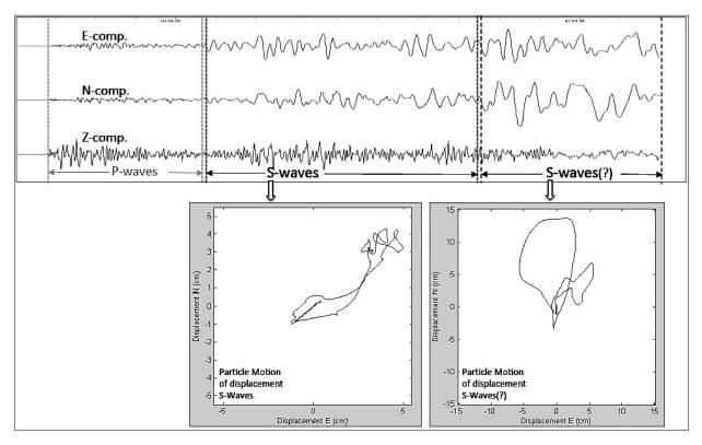
**Figure 11.** Displacement particle motion at the DURR station estimated for the first S-wave window and the second stronger part of S-wave(?) window of the mainshock.
