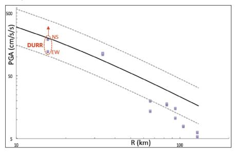
**Figure 2.** Comparison of recorded PGAs of the Non. 26, 2019 earthquake (M6.4) with a regional GMPE of Skarlatoudis et al. (2003) (solid line:mean, dashed lines:1sd).
