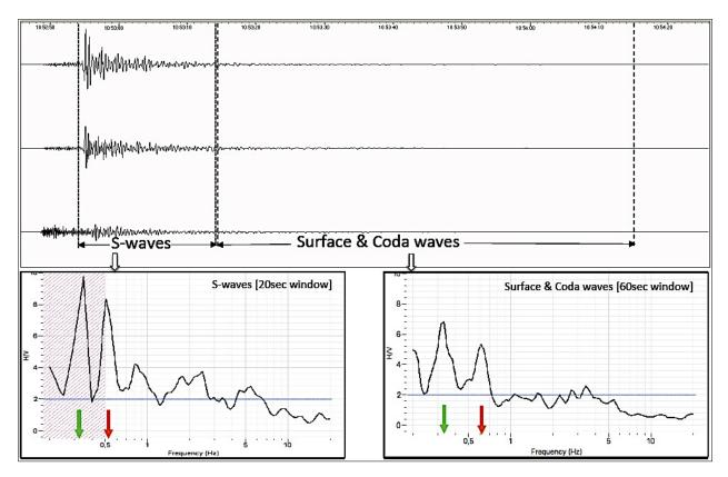
**Figure 14**. Horizontal-to-Vertical Spectral Ratio (HVSR, Receiver Function) at the DURR station estimated for the S-wave window and the surface & coda waves window of the aftershock of 28/11/2019, 10:52:44 (M4.6).
