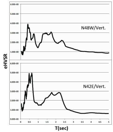
**Fig. 10.** Earthquake Horizontal-to-Vertical spectral ratio for both horizontal components based on the 5% damped response spectra at the SMG1 station.
