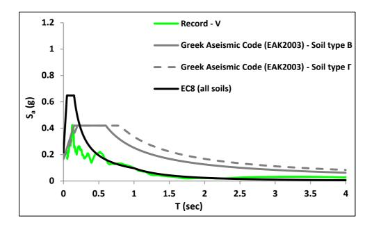
**Fig. 9.** Comparison of the 5%-damped elastic acceleration response spectra between the earthquake record in Vathi, Samos and the Greek Seismic codes (EAK2003 and EC8): Vertical component of seismic motion.
