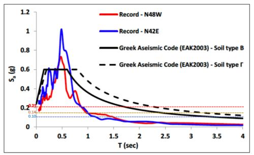
**Fig. 7.** Comparison of the 5%-damped elastic acceleration response spectra between the earthquake record in Vathi, Samos and the Greek Aseismic Code (EAK2003): Horizontal components of seismic motion. The horizontal lines anchored at 0.10, 0.14, 0.21g show base shear coefficients according to 1959 Greek Seismic Code for ultimate strength design.
