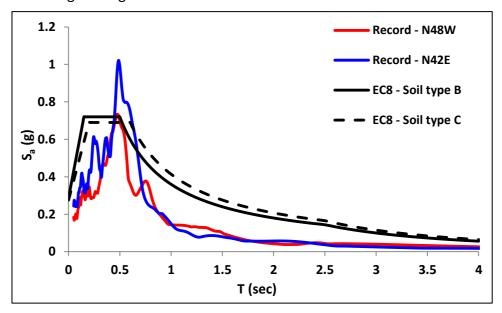
**Fig. 8.** Comparison of the 5%-damped elastic acceleration response spectra between the earthquake record in Vathi, Samos and the EC8 Code: Horizontal components of seismic motion.
