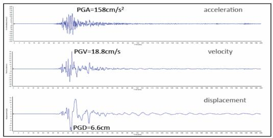
Fig. 3. Time histories of the horizontal component (direction N48W).
